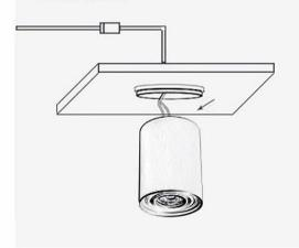
4. The rotating lamp body engages with the bottom part.
