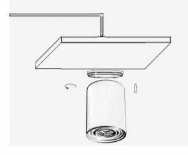
2. Secure the bottom part to the ceiling.
