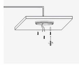
3. Connect the cable with connector.
