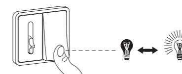
**Dimming the load**
